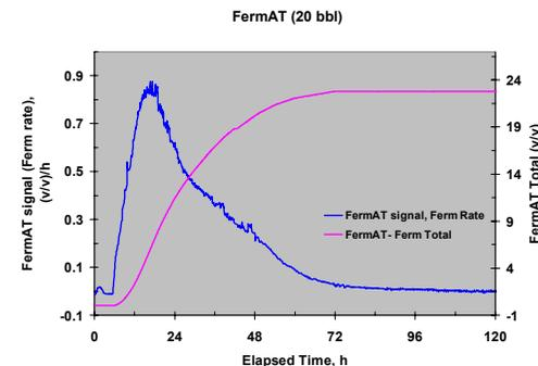
Fig 2. Another example fermentation fingerprint. A faster specific fermentation rate as well as smaller fermentation volume substantially relieved  $CO_2$  supersaturation.
