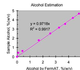
Fig 4a. Typical goodness-of-fit: Alcohol determined by FermAT agrees closely with values determined with off-line analyses.
