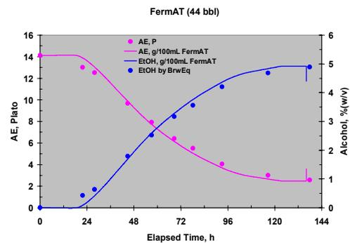
Fig 3. Continuous monitoring of the fermentation of Fig.1 for alcohol production and extract attenuation in real-time. Symbols represent traditional off-line measurements from grab-samples.
