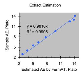
Fig 4b. Typical goodness-of-fit: Extract determined by FermAT agrees closely with values determined with off-line analyses.
